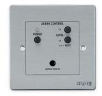
ACPR is a wired remote control with local line input for the Apart SDQ5PIR active speaker. The ACPR audio control panel has a line input at the rear on euroblock connectors and one 3.2 mm stereo jack input on the front panel. This rear line input is in use when no jack is inserted in the front panel jack connector. Inserting a jack automatically disables the rear line input.
